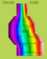
The cross section above shows how the multi-chambered profile prevents the transfer of heat from the inside to the outside
